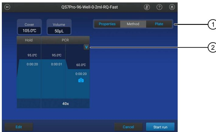
① Indicates that this is the **Method** tab where the VeriFlex™ Zones settings can be removed
