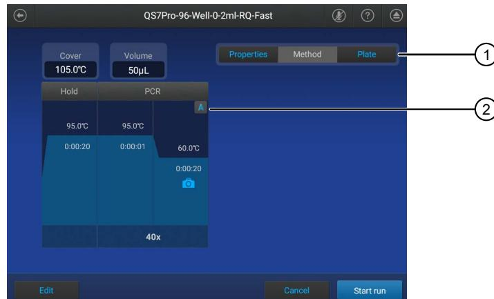
① Indicates that this is the **Method** tab where Auto Delta settings can be removed.
